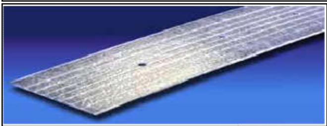
Figure 2. Coupon Condition (Before Burial of Coupon in Soil Samples)
