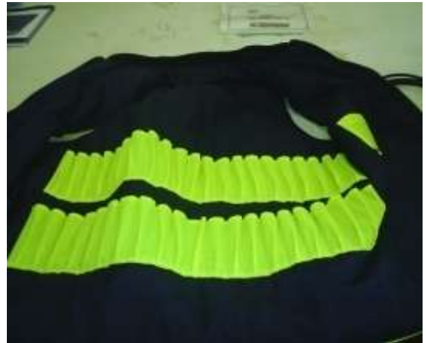
Fig.1. The customized vest for holding of waste samples and wear on the human body for incubation
