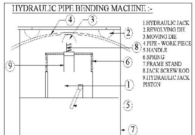
Fig. 1. Design details of Hydraulic Pipe Bending Machine
