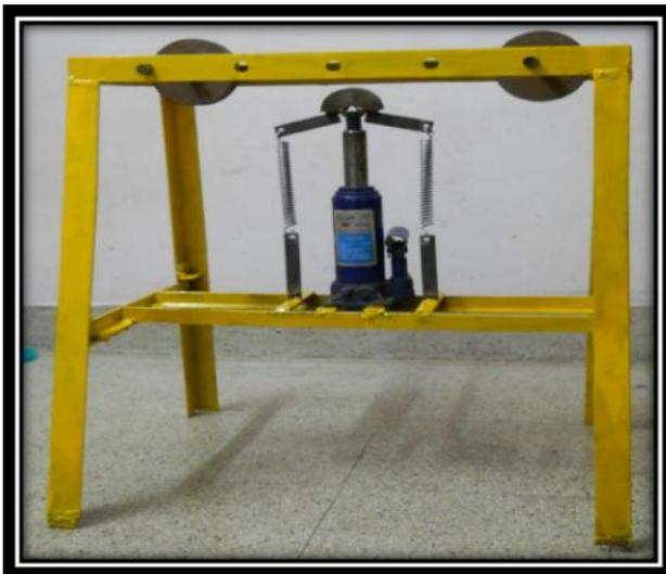
**Fig. 2. Fabricated Hydraulic Pipe Bending Machine**
