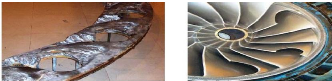
Cracking and breakage of runner vanes at outlet
