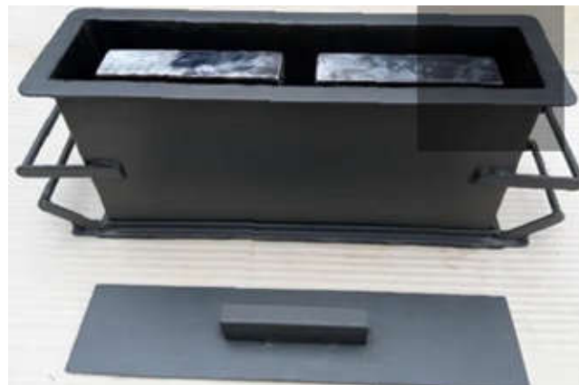
Figure 3. Form for production of concrete blocks
