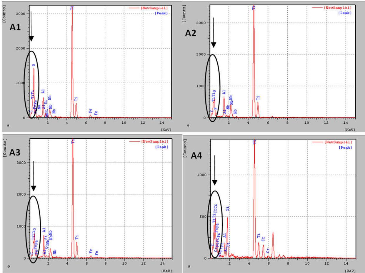
Figure 2. EDS analysis coupled to the SEM for samples treated by NGC technique
