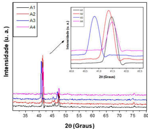
Figure 3. X-ray diffraction of the TiN film
