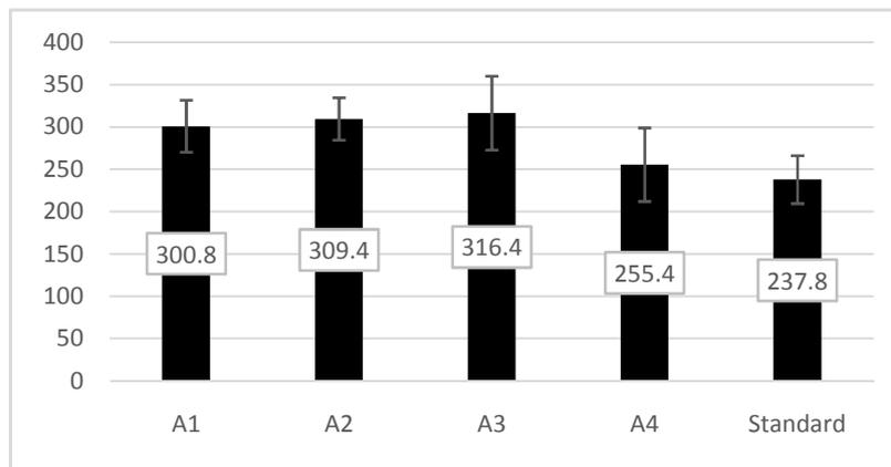
Figure 5. Vickers microhardness values for CCN treatment conditions A1, A2, A3 and A4
