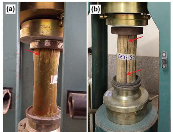
Figure 9. Rupture of (a) bamboo without concrete and (b) with concrete filling
