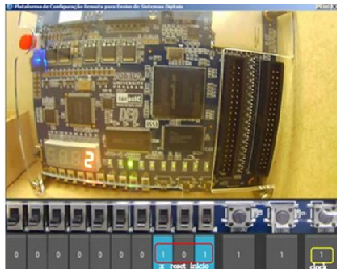
Figure 13. Remote platform operation, test of the sequential circuit (sequence "101")
