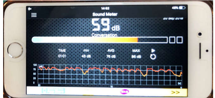
Figure 1. Image of the reading of the mobile device with application "decibel meter", presenting the graph of sound measurement, with a minimum, maximum and average value of dB with the 1 minute recording period of the child's crying
