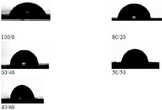
Figure 3. Droplet photos: contact angle between water and WPCs (rHDPE/sawdust) surface
