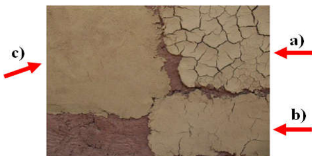
Figure 3: The figure illustrates the effects of adding sand to earth mortar. The trace a) has not sand addition; the trace b) has low sand addition; and the trace c) has biggest sand addition and less shrinkage. Fonte: Santos, (2015)
