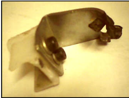
Fig. 3. Broken Pu –Material with Shifter Fork
