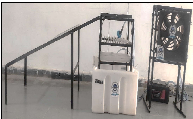
Fig. 5. Solar Evaporative cooling system
