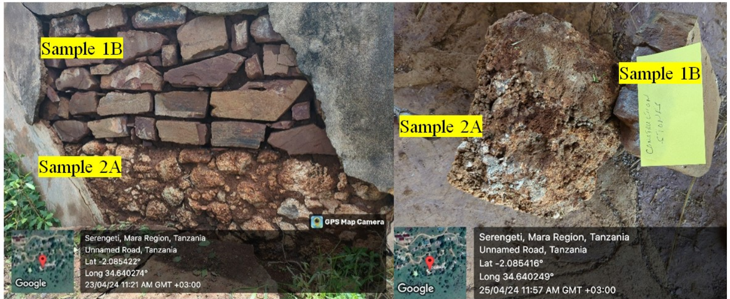
Figure 2. Identified two different natural stone samples used for the construction of the Fort Ikoma historical building in SENAPA, Tanzania
