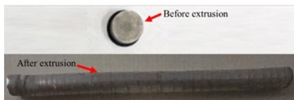
Figure 2. Aluminum Alloy before and after extrusion
